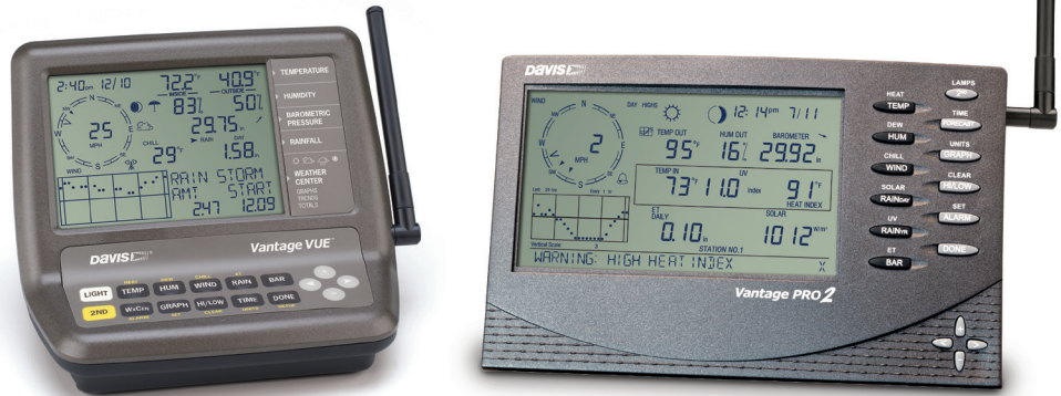
Use your console as a repeater to transmit data from one console/receiver to another.
